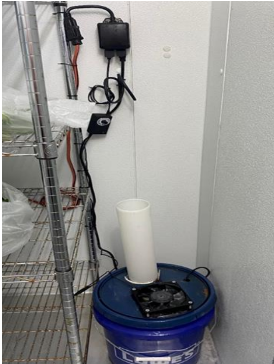
Figure 5. Our humidifier with a white plastic PVC tube in the lid adjacent from the fan, so the mist would then leave the bucket into the cooler.
