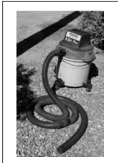
Figure 2. A standard shop vacuum used for sucking-up seed and detaching the seed from floral structures.
