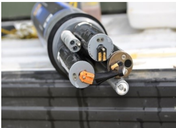
Figure 1. A multiprobe Sonde set to continuously monitor water quality.
