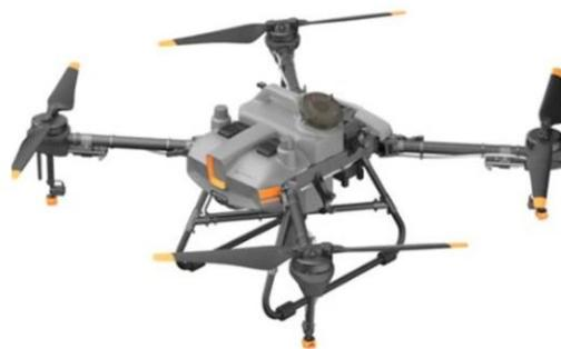
Example: DJI Agras T10 bundle: \$14,000; 2.1 gal tank (18 lbs water); 18 ft ESW; frame 29 lbs
