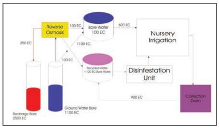
Figure 2. Flow diagram of alternative irrigation system.
