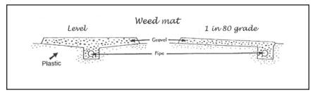
Figure 2. Floor construction in our production areas.
