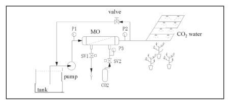
**Figure 1.** A view showing an example of plant-growing apparatus in the present paper. The apparatus is roughly made up of, from the upstream side, a water tank, a pressure pump, a hollow fiber membrane module MO, a  $CO_2$  gas cylinder, a control valve SV2, and a relief valve. Operations of the entire apparatus are controlled by a control unit (not shown).
