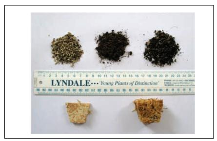
**Figure 1.** Media: Left to right (top row): pumice (3–5mm), peat, 90% pumice : 10% peat, (bottom row) compressed sphagnum, and expanded sphagnum.
