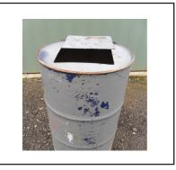
**Figure 2.** The flap cut from the top of the drum to adjust the amount of light entered.
