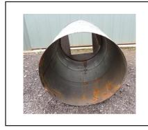
**Figure 1.** The 250-L drum with the base cut out.
