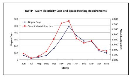
Figure 2. Comparison of daily electricity cost at British Wild Flower Plants (£ per day) against the requirement for space heating (degree days) from June 2010 to May 2011.
