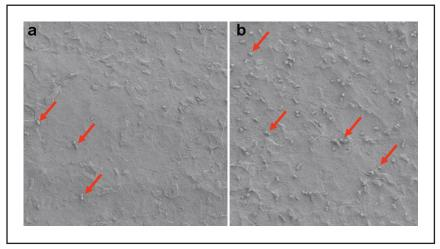
**Figure 1.** Scanning electron microscopy (SEM) image of titanium surfaces immersed in (A) ferrous ferric chloride (FFC) or (B) control solutions for 4 days. Prior to immersion SEM images showed clean surfaces. Image size:  $40 \times 40 \ \mu\text{m}^2$ .
