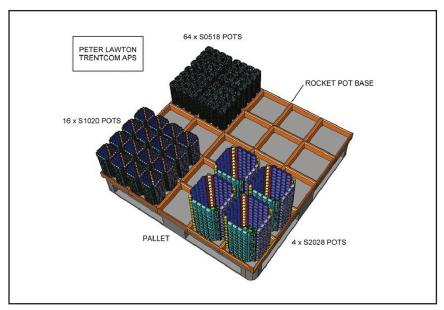
Figure 5. A 3D computer graphic of the new pot proposal. Three new pots are shown on a new pallet.
