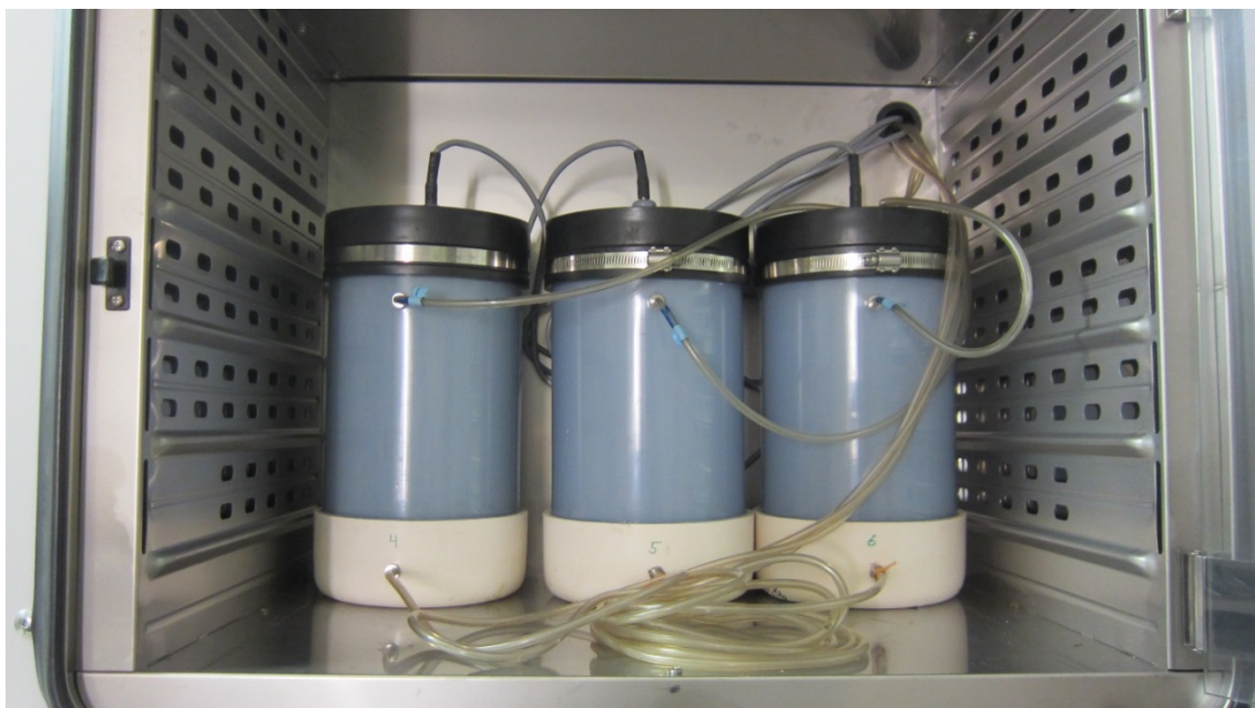
Fig. 2. Three bioreactors inside of a high-temperature incubator. The system consists of three incubators, allowing for the simultaneous operation of nine bioreactors. Humidified air enters the reactor at the bottom, and exits the top. The reactors hold approx. 4 L and are constructed with 15.2 cm diameter PVC.
