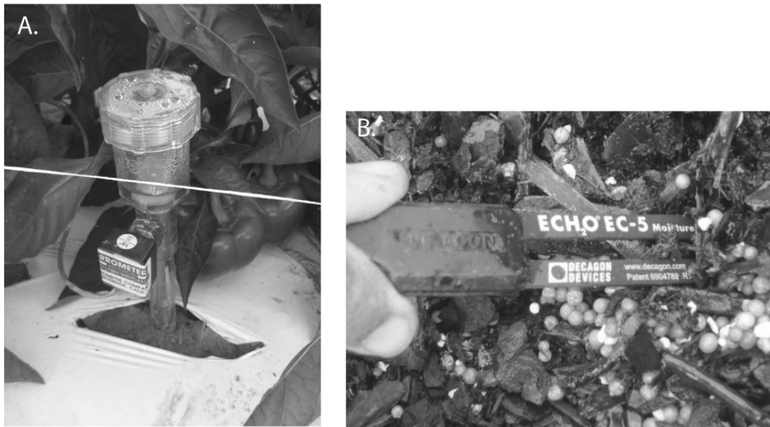
Fig. 4. Substrate moisture sensors (A) tensiometer, and (B) electrical resistance sensor.
