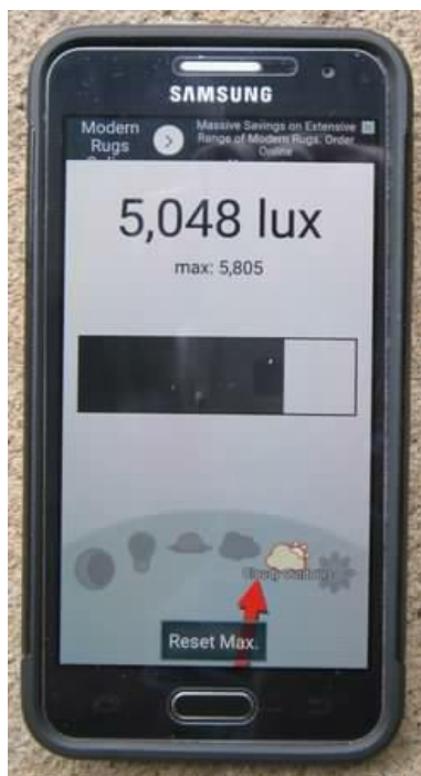
Light-O-meter App for measuring light levels under shade cloth or determining need for supplemental lighting
